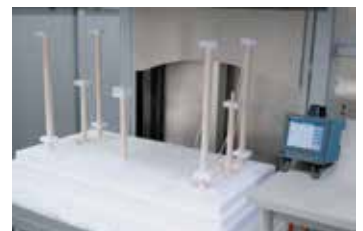
Measurement setup to determine the temperature uniformity in a high-temperature lift-bottom furnace
