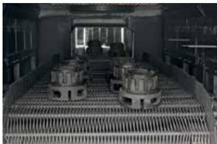
Mesh belt drive in a continuous furnace
