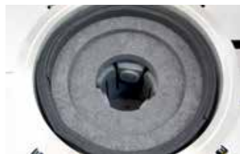
Graphite heating module
