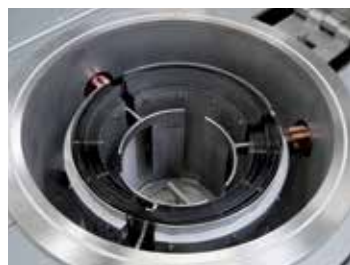
Cylindrical retort with tungsten heating
