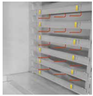
Adjustable plate shutters to adapt the air guide to the charge
