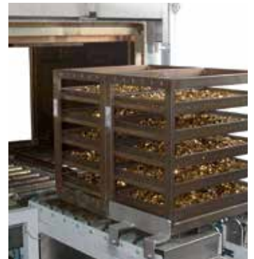
Continuous furnace for bulk materials in baskets
