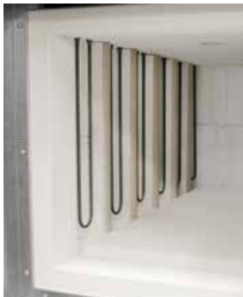
Protection of heating elements against mechanical damage
